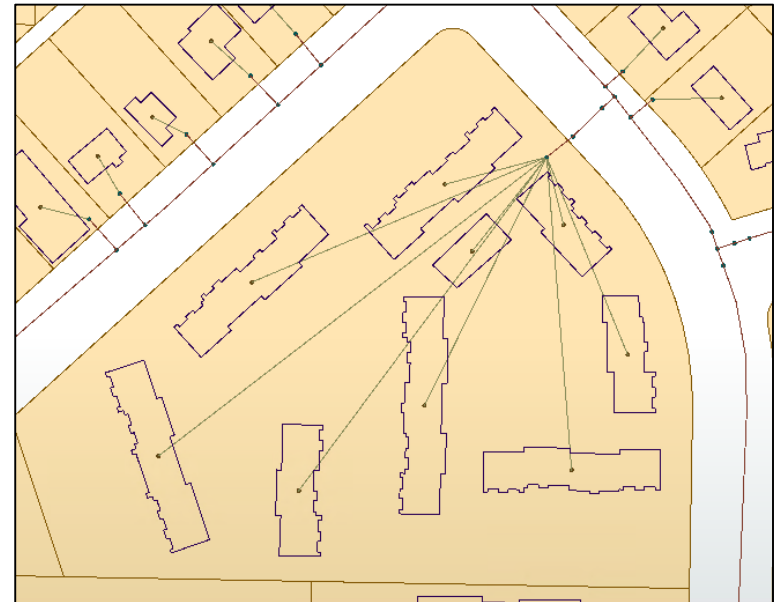
An instance of many buildings, all from the same parcel having their TerminalElement Nodes connected to the NetworkGraph at the same service line node. Picture from FME Data Inspector.
