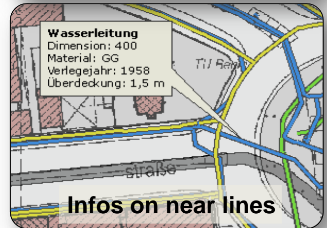
Crossing utility lines
